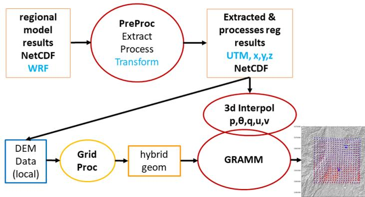
**Figure 2.** Schematic of the data flow regional-local and related processing and interfaces.
